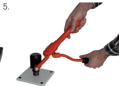
Pilot hole - For bolt Ø 9.5 mm, with Ø 10.5 mm - For bolt Ø 11.1 mm, with Ø 12 mm - For bolt Ø 19 mm, with Ø 20 mm, for bolt Ø 19 mm you can also pre-drill a Ø 20.4 mm hole - For shaped punches: use largest bolt diameter + 1.5 to 2 mm
